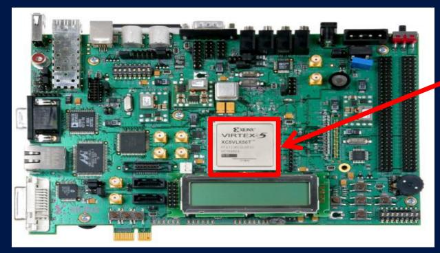
Embedded system on a Xilinx Virtex 5 FPGA.
